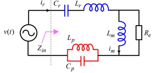
Fig. 4. Simplified circuit of a multi-resonant converter.
