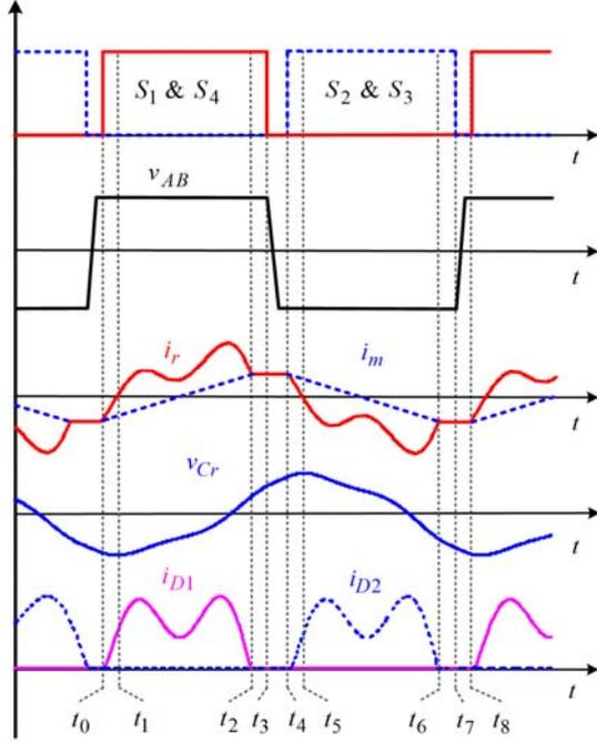
Fig. 3. Typical waveforms of a multi-resonant converter below the resonant frequency  $f_{r1}$ .
