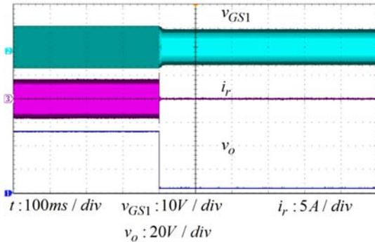
(b) Waveforms during the short output protection.
