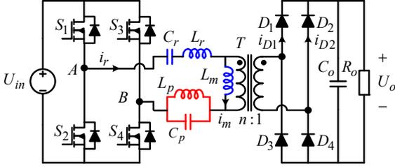
Fig. 1. Topology of a multi-resonant converter.
