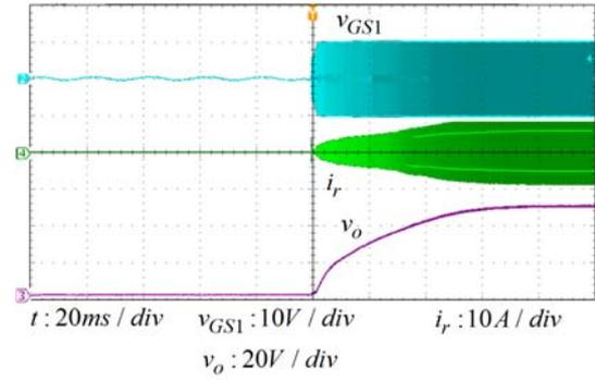
(a) Waveforms during the start-up condition.
