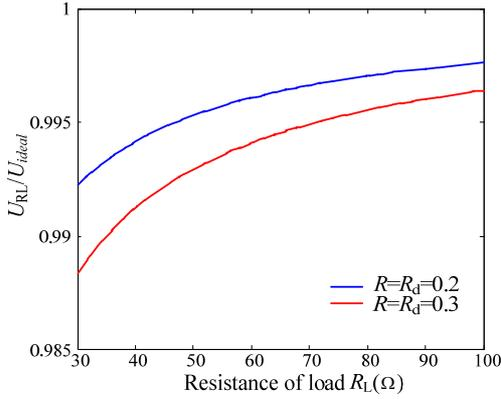
Fig. 6. Effect of the inner resistances on the output voltage in the LCL-S topology.
