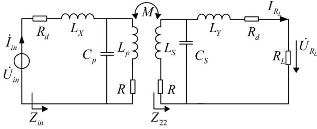
Fig. 3. LCL-LCL topology considering the inner resistances.
