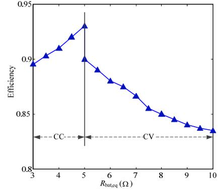
Fig. 10. Measured efficiencies during the charging process.
