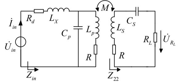
Fig. 4. LCL-S topology considering the inner resistances.
