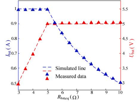
Fig. 9. Charging profile during the whole charging process.
