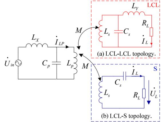
Fig. 2. Equivalent circuits of WPT systems with different compensation topologies.
