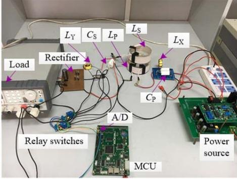
Fig. 8. Experiment prototype of a WPT battery charger.
