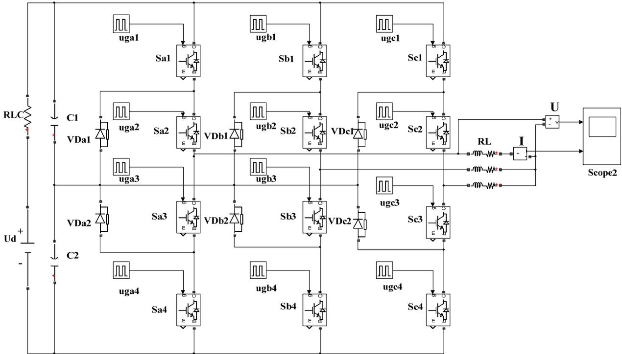
Fig. 5. Simulation model of the Three-Level NPC inverter.
