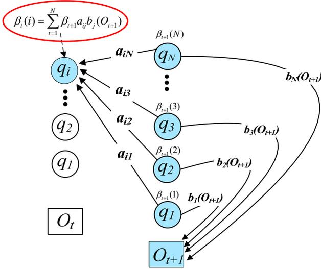
Fig. 2. Procedure of Backward algorithm.
