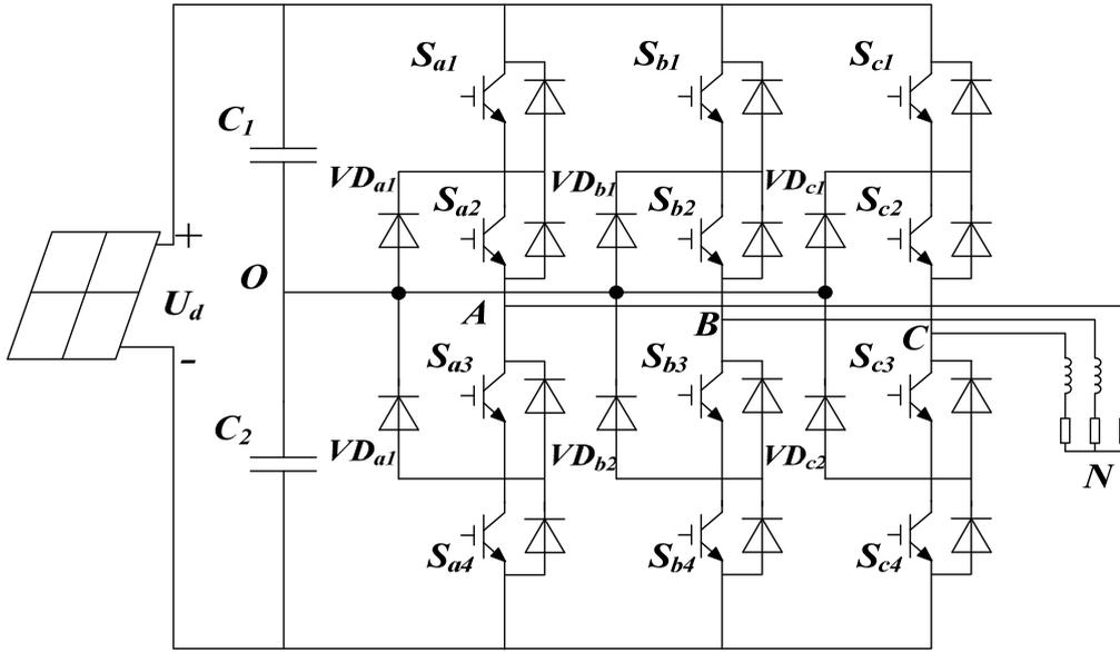
Fig. 1. Topology of Neural-Point-Clamped photovoltaic inverter
