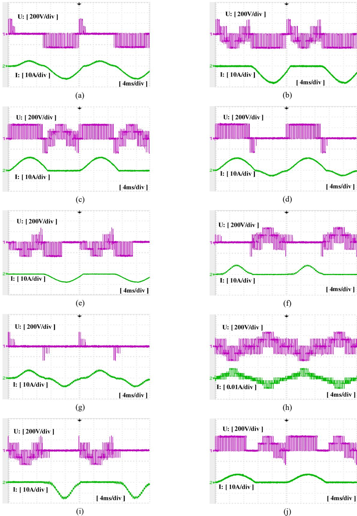
Fig. 9. Experimental waveforms in each fault state.(a) Fault number 1, (b) fault number 2, (c) fault number 3, (d) fault number 4, (e) fault number 5, (f) fault number 6, (g) fault number 7, (h) fault number 8, (i) fault number 9, (j) fault number 10.
