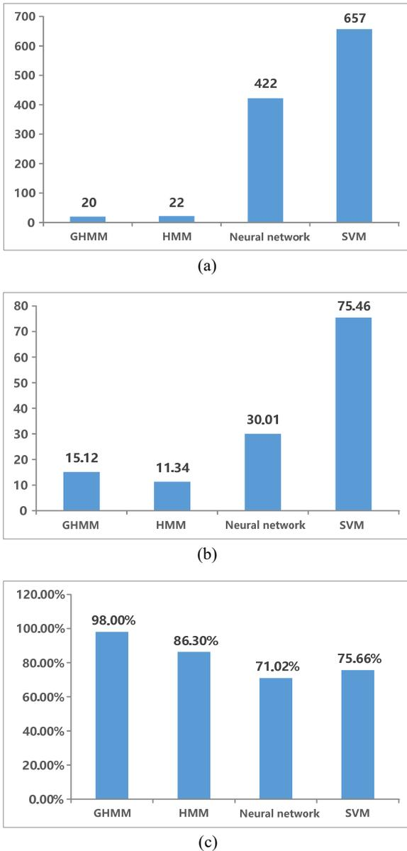
Fig. 7. (a) Average iterative steps, (b) average training time(s) and (c) correct recognition rate.
