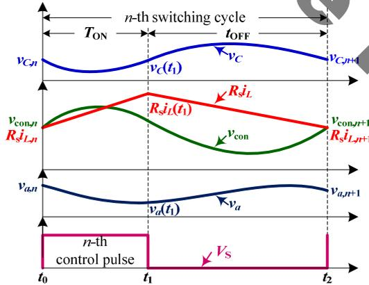
Fig. 3. Main steady-state operation waveforms in the  $n$ -th switching cycle.
