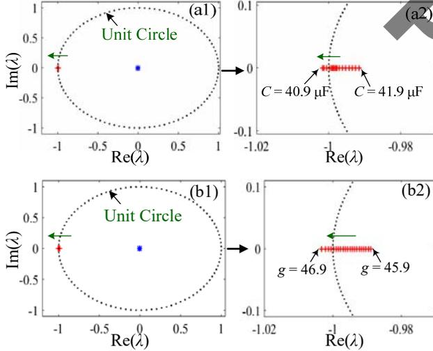
Fig. 5. Loci of two eigenvalues for the converter, where “\*” and “+” denote  $\lambda_1$  and  $\lambda_2$ , respectively: (a)  $C$  decreasing from 41.9  $\mu\text{F}$  to 40.9  $\mu\text{F}$ ; (b)  $g$  increasing from 45.9 to 46.9; (a2) and (b2) are close-up views of the eigenvalue  $\lambda_2$  in (a1) and (b1).
