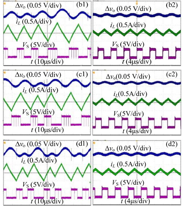
Fig. 7. Experimental results for different circuit parameters  $g$ ,  $C$ ,  $r$ ,  $R_s$  and  $T_{ON}$  listed in Table II, where  $\Delta v_o$ ,  $i_L$  and  $V_s$  denote output voltage ripple, inductor current and control pulse voltage, respectively.
