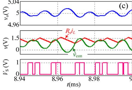
Fig. 2. Stable operation and subharmonic oscillation in a COT-CMC buck converter with a PI compensator: (a)  $C = 47 \mu\text{F}$  and  $g = 40$ , stable operation; (b)  $C = 30 \mu\text{F}$  and  $g = 40$ , subharmonic oscillation; (c)  $C = 47 \mu\text{F}$  and  $g = 60$ , subharmonic oscillation.
