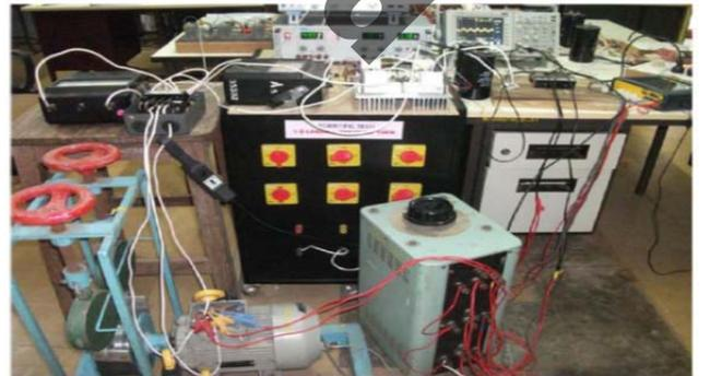
Fig. 4: Experimental setup of a 3 phase 2 level SVPWM controlled VSI.
