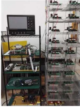
Fig. 9. Photo of a single-phase MMC prototype.
