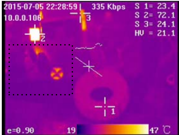
Fig. 17. Thermal image showing the heat dissipation in the PCS during 1kW operation S1=Boost coupled inductor transformer, S2=Boost diode, S3= Boost switch S_b , marked area= diodes and capacitor of the charge-pump.
