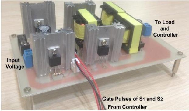
Fig. 8. Photo of the power section of the prototype.
