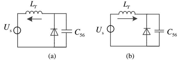
Fig. 9. High-frequency diode equivalent circuit. (a) Diode forward-conduction equivalent circuit. (b) Diode reverse-blocking equivalent circuit.
