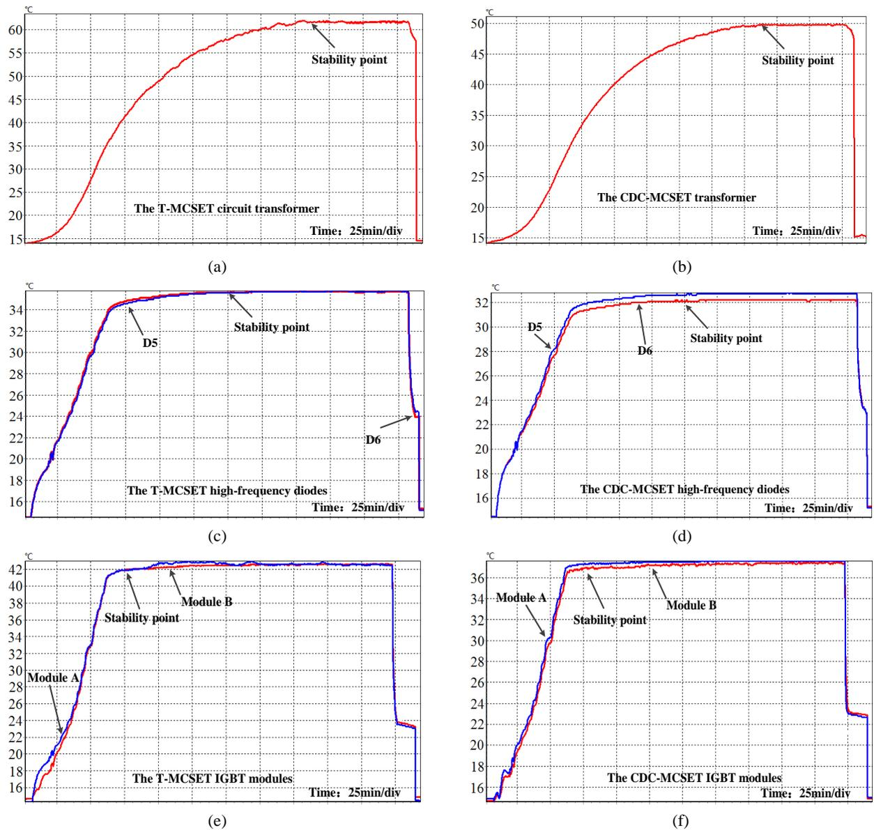
Fig. 16. Temperature curve of the MCSET key components.
