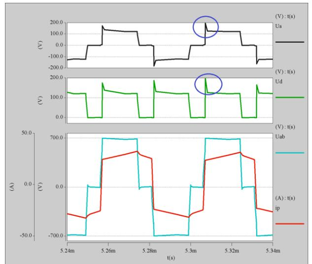
Fig. 11. T-CSC simulation waveform.  $U_s$  is the secondary voltage waveform of the transformer,  $U_d$  is the high-frequency diode output voltage waveform,  $U_{ab}$  is the primary voltage waveform of the transformer between “a” and “b,” and  $i_p$  is the primary current waveform of the transformer.
