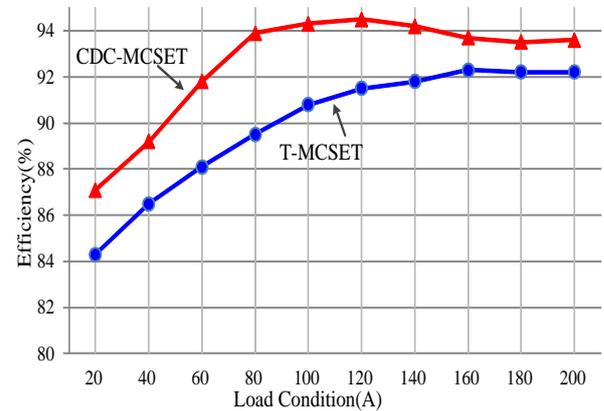
Fig. 19. Comparison of efficiency and load current.
