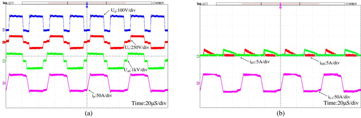
Fig. 15. CDC-MCSET physical waveform. (a)  $U_d$  is the high-frequency diode output voltage waveform,  $U_s$  is the secondary voltage waveform of the transformer,  $U_{ab}$  is the primary voltage waveform of the transformer between “a” and “b”, and  $i_p$  is the primary current waveform of the transformer. (b)  $i_{D7}$  is the diode  $D_7$  current,  $i_{D8}$  is the diode  $D_8$  current, and  $i_{L1}$  is the resonant inductor  $L_1$  current.
