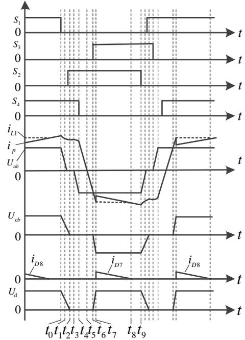
Fig. 6. Clamping-diode controlled-source circuit waveform.
