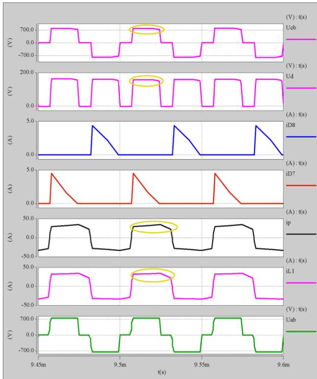
Fig. 12. CD-CSC waveform.  $U_{ab}$  is the primary voltage waveform of the transformer between “c” and “b”,  $U_d$  is the high-frequency diode output voltage waveform,  $i_{D7}$  is the diode  $D_7$  current,  $i_{D8}$  is the diode  $D_8$  current,  $i_p$  is the primary current waveform of the transformer,  $i_{L1}$  is the resonant inductor  $L_1$  current, and  $U_{ab}$  is the primary voltage waveform of the transformer between “a” and “b.”
