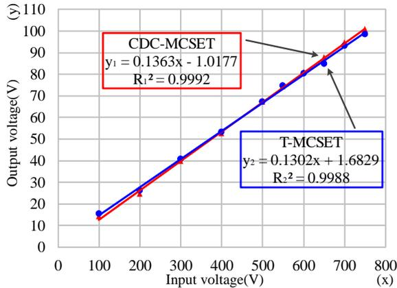
Fig. 17. Comparison of output voltage  $U_o$  and input voltage  $U_{in}$ .
