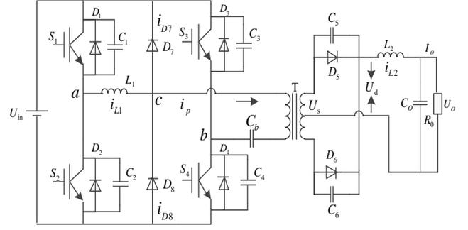
Fig. 5. Clamping-diode controlled-source circuit.
