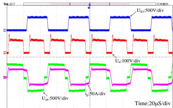
Fig. 14. T-MCSET physical waveform.  $U_d$  is the high-frequency diode voltage,  $U_{S3}$  is voltage waveform of the lagging switch  $S_3$ ,  $U_{ab}$  is the primary voltage waveform of the transformer, and  $i_p$  is the primary current waveform of the transformer.
