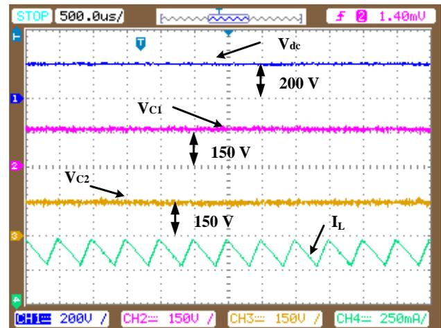
Fig. 20. Experimental waveforms of the input voltage, output capacitor voltages and inductor current of a three-level boost converter (capacitor voltage 150V/div, input dc voltage  $V_{dc}$  200V/div, inductor current 250mA/div).
