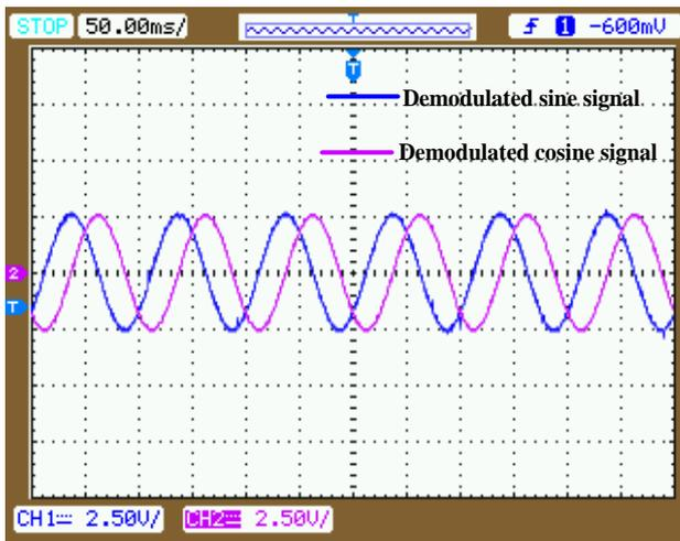
Fig. 17. Experimental results of a demodulated sine and cosine signal.
