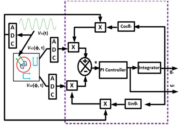
Fig. 5. Schematic of the RDC-less position estimation.
