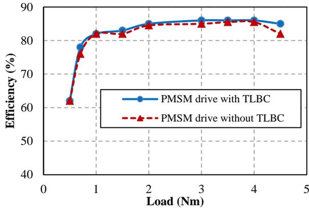
Fig. 25. Efficiency of the proposed PMSM drive.
