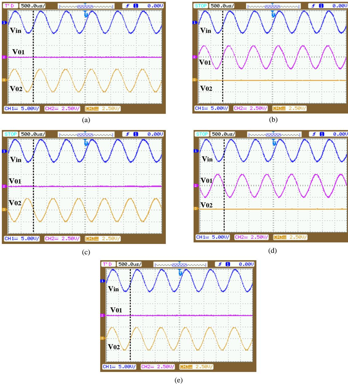
Fig. 15. Experimental results of the resolver output signal at: (a)  $0^\circ$  shaft rotation, (b)  $90^\circ$  shaft rotation, (c)  $180^\circ$  shaft rotation, (d)  $270^\circ$  shaft rotation, (e)  $360^\circ$  shaft rotation.
