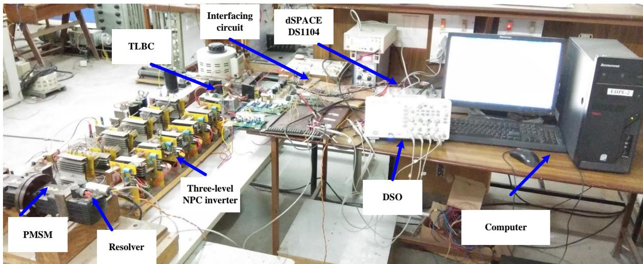
Fig. 14. Experimental setup.
