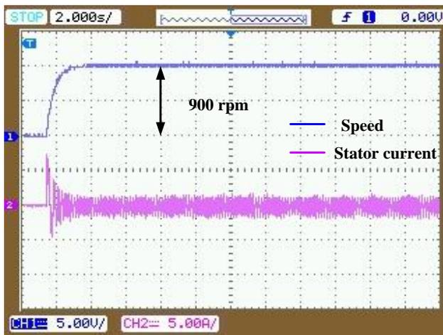
Fig. 22. Experimental result of the starting response of a PMSM drive (speed 450 rpm/div and stator current 5A/div).
