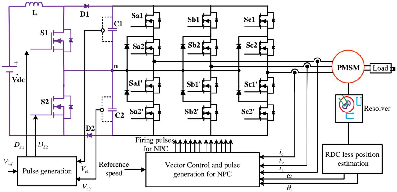
Fig. 1. Schematic diagram of the proposed PMSM drive system.
